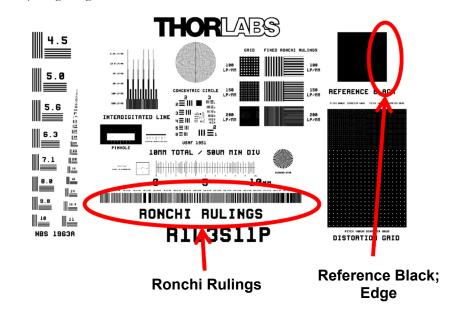
**Figure 1:** Location of Ronchi rulings on the resolution target. Largest line spacing (10 lp/mm) is on the far left; smallest (200 lp/mm) is on the far right. The 'Reference Black' area is also shown; use the edge indicated for finding the MTF using the edge-spread function.
