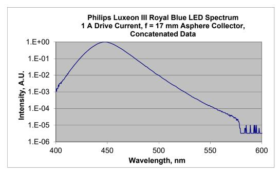
Figure 2. Spectrum of our blue LED; only relative intensity was measured, hence the units on the Y-axis are arbitrary (Arbitrary Units).
