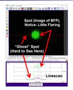
Figure 3: BFP spot appearance on the color camera when properly aligned.
