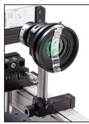
Figure 2: Aluminum foil strip blocking center of the aperture stop.
