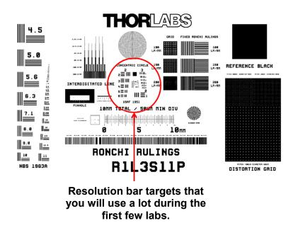
**Figure 2:** Thorlabs custom resolution target R1L3S11P, showing the USAF 1951 3-bar resolution target area. On the left are the 5-bar resolution elements (NBS1963A standard; NBS stands for 'National Bureau of Standards', the predecessor of NIST, the National Institute of Standards and Technology). The USAF target is more convenient since the elements spiral in to the center as the spacing goes down, so you can see more sizes at once.
