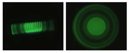
**Figure 1:** Phase rings in BFP of objective. Left: standard image. Right: with a diffuser (a Kimwipe, held just in front of the field stop) to aid in filling the entire AS with light. The darkest ring is the phase ring; the lighter rings inside and outside the main dark ring are "apodizing" rings, designed to help reduce the "halo" effect typical of phase contrast images.
