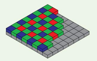
**Figure 1:** A Bayer array featuring RGB filters on top of an underlying monochrome sensor. Image after Wikipedia (2006).
