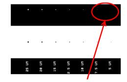
Use these smallest holes (7.5 and 5.0 µm diameter).
