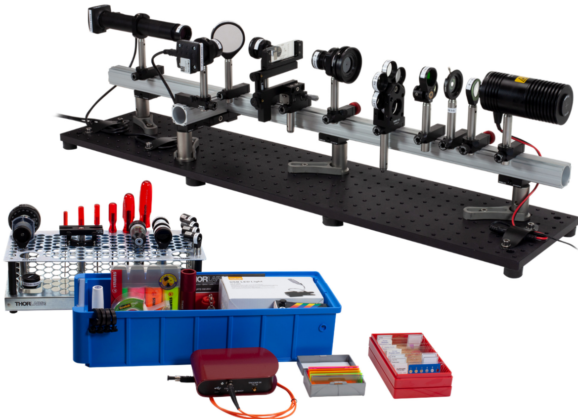
Figure 1 Overview of the optical microscopy setup. The kit contains an open rail with all optical components to go through the teaching steps. Furthermore the kit contains a research grade spectrometer, various samples and tools to experiment, learn and evaluate.
