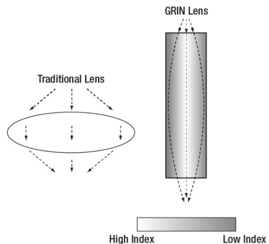
**Figure 1. GRIN Lens vs. Singlet.** A gradient lens has an index of refraction gradient orthogonal to its optical axis. This gradient bends light inside of the lens. This bending of light can mimic the focusing ability of traditional singlet lenses, where light is bent by the external shape of the lens and the refractive index change between the lens and the surrounding air.
