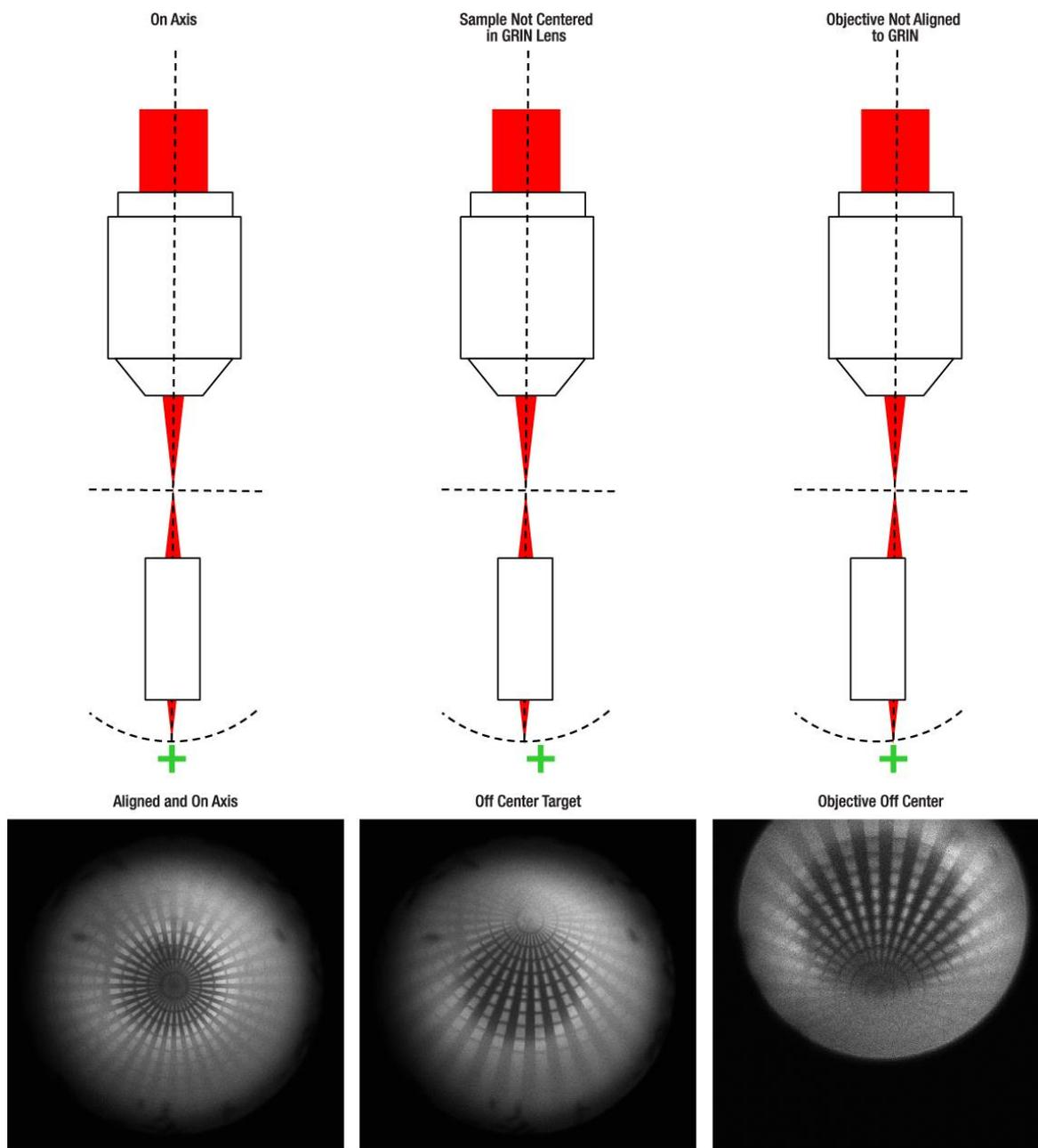
**Figure 5. GRIN Lens Imaging Target On and Off Axis.** Thorlabs Star Target (R1L1S1P) imaged through fluorescein, a Thorlabs GRIN lens (G1P11), using a Bergamo® multiphoton microscope. The curvature in the imaging field curves the imaging plane away from the target. The resolution is best in the center of the GRIN lens FOV and moving the microscope objective in Y or Z does not recover the resolution lost at the edges of the GRIN FOV.
