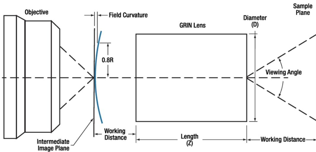
**Figure 3. GRIN Lens and Imaging Objective.** A GRIN lens aligned with an imaging objective. GRIN lenses’ imaging properties include working distance, field curvature, and viewing angle.
