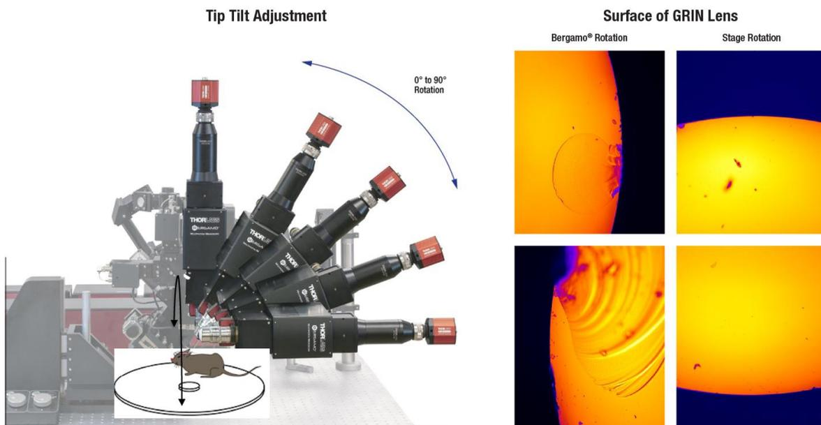
**Figure 7. GRIN Lens Alignment.** By carefully adjusting the angle of the microscope and the animal stage, the GRIN lens can be exactly aligned with the objective. In this example (left), the GRIN lens is rotated by adjusting the animal in one axis, and the Bergamo® rotation microscope is rotated in the orthogonal axis. Alignment is checked by imaging the top surface of the GRIN lens (right), to make sure all edges are in focus.
