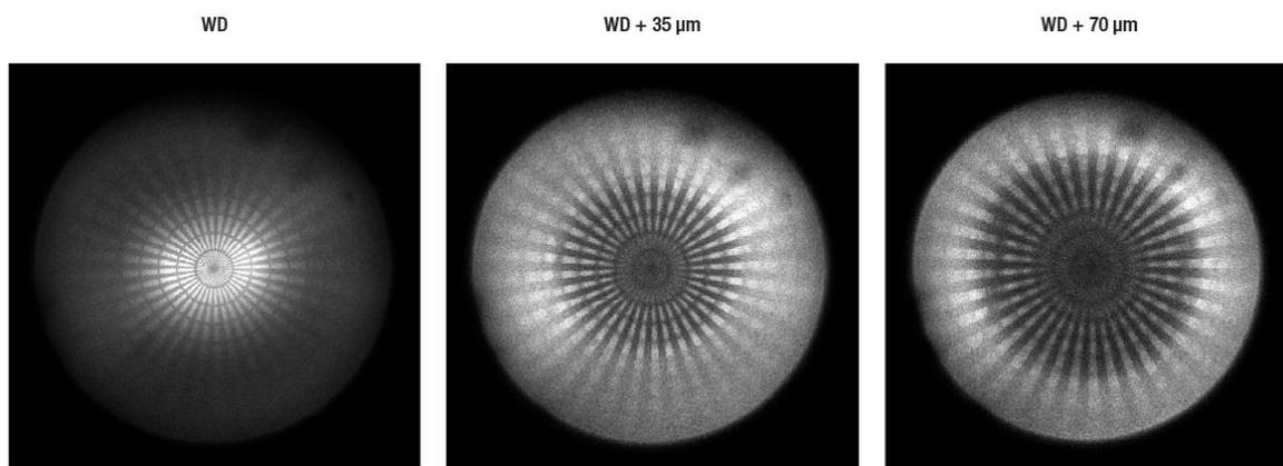
**Figure 10. GRIN Lens Field Curvature.** Thorlabs Star target imaged through fluorescein and a 1 mm diameter, 9 mm long GRIN lens. This high pitch GRIN lens introduces significant optical aberrations, including field curvature. Since the field curves toward the GRIN lens, one must focus deeper to image the same focal plane off axis  $WD =$  Working distance. A flat field would have roughly equal brightness rather than a spot or ring.
